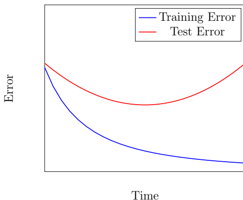
Figure 4: The optimal place to stop the network’s training would be at the minimum of the red curve.
